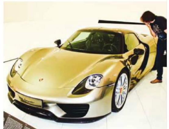
The 2014 Porsche 918 Spyder Hybrid used a mid-mounted 4.6-litre V-8 and twin electric motors to hit 60 mph in less than three seconds, and run the quarter-mile in 9.8 seconds. It stickered for about $850,000.
