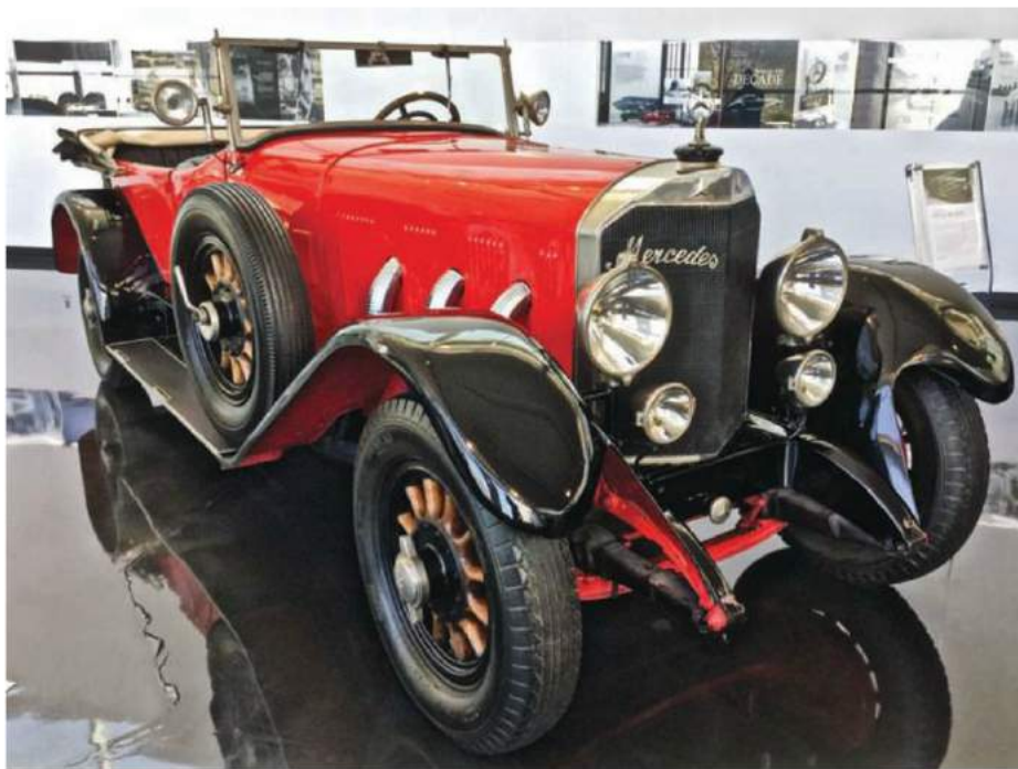
A 1927 Mercedes-Benz 630K 24/100/140 PS at the Mercedes-Benz Visitors Center. Power came from a supercharged 140-hp inline six.
